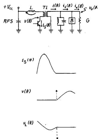
Fig. 11. Parallel-tuned class E amplifier with series inductor.
