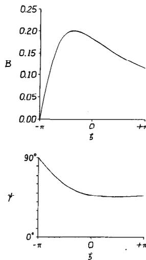
Fig. 3. Circuit element values for 100-percent efficiency with 50-percent duty cycle ( $R=1$ ).
