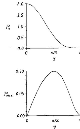
Fig. 8. Power output as function of duty cycle ( $R=1, V_{cc}=1$ ).
