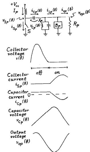
Fig. 12. Parallel-tuned class E amplifier with series capacitor.
