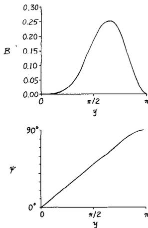
Fig. 6. Circuit element values for 100-percent efficiency with different duty cycles ( $R=1, \zeta=0$ ).
